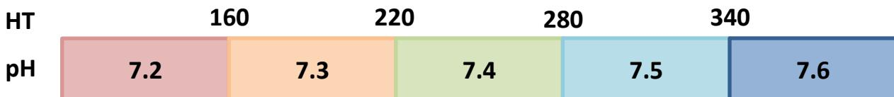
These values stem from our experience. They are recommended to preserve the elements in contact with water and the correct functioning of the measuring probes.
